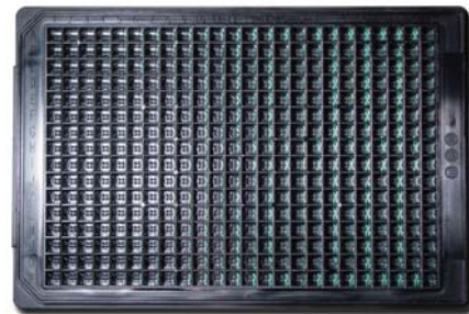
Multi-Spot 384-well Plate with 4 spots per well
