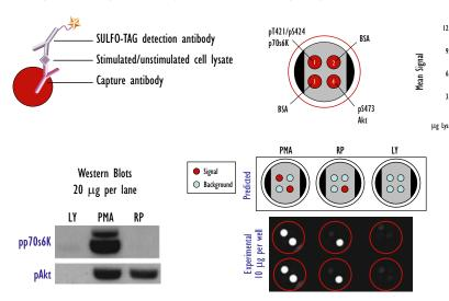
Logarithmically growing Jurkat cells were treated with LY, Rapamycin, and PMA. Whole cell lysates were added to MSD MULTI-SPOT® 4 Spot 96-well High Bind plates coated with capture antibody at two of the four spatially distinct electrodes per well. Phosphorylated proteins were detected with MSD SULFO-TAG<sup>TM</sup> detection antibodies.
