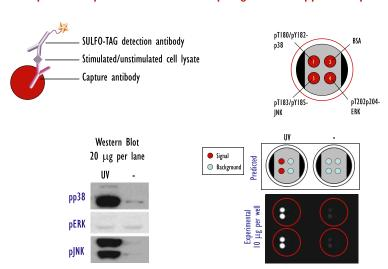
Logarithmically growing HEK293 cells were treated +/- UV. Whole cell lysates were added to MSD MULTI-SPOT 4 Spot 96-well High Bind plates coated with capture antibody at three of the four spatially distinct electrodes per well. Phosphorylated proteins were detected with MSD SULFO-TAG detection antibodies.
