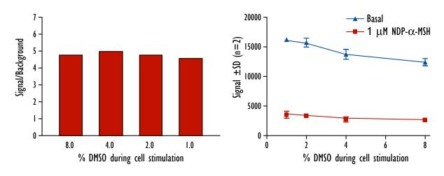
Cells (5,000/well) were challenged with buffer or 1  $\mu$ M NDP- $\alpha$ -MSH in the presence of increasing concentrations of DMSO. The assay tolerates DMSO at final concentrations of up to 8% without significant change in the signal to background ratio.
