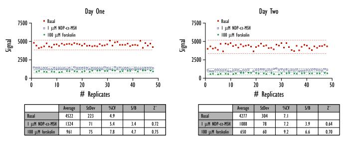
The accumulation of cAMP in response to NDP- $\alpha$ -MSH and, separately, forskolin was compared to unstimulated cells (basal) according to the protocol. The high Z' scores reveal that the assay is robust within an HTS workflow.
