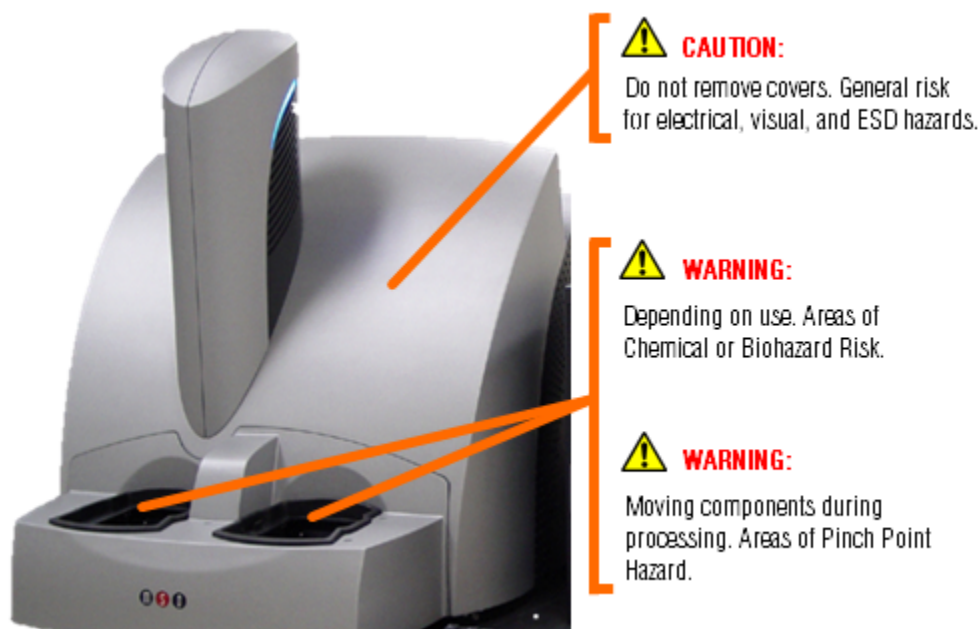
Figure 2:1 SECTOR Imager electrical hazards. SECTOR Imager 6000 shown.
