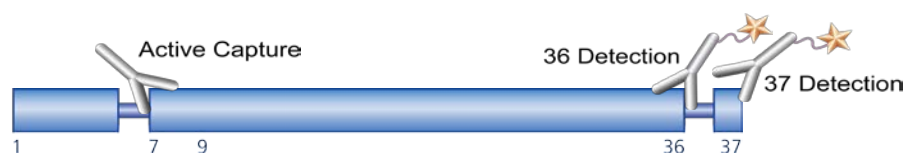
Figure 2. Schematic of the antibodies recognition sites for the Total Active GLP-1 Assay on GLP-1 protein amino acids 1-37.
