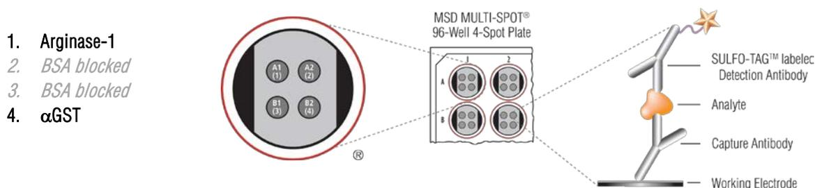
**Figure 1.** Spot diagram showing placement of analyte capture antibody. The numbering convention for the different spots is maintained in the software visualization tools, on the plate packaging, and in the data files. A unique bar code label on each plate allows complete traceability back to MSD manufacturing records.
