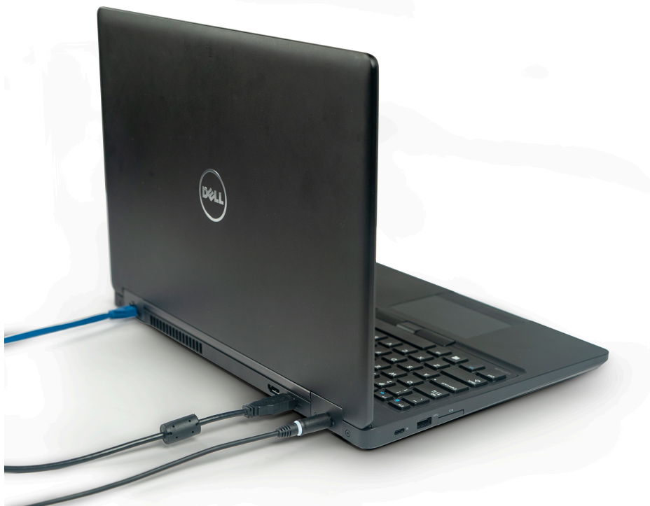
FIGURE 2.6. Laptop computer cable attachments (Ethernet, USB, and power).
