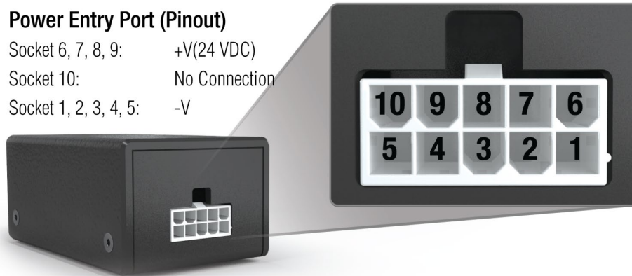
FIGURE 2.5. The electrical noise filter.
