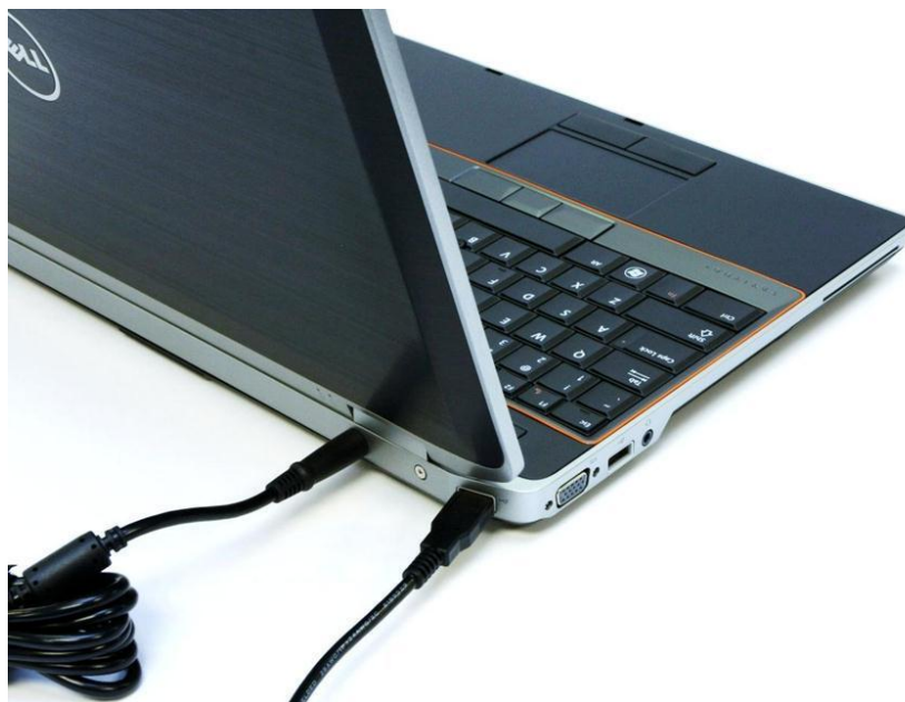
Figure 3:8 Notebook computer cable attachments (USB and power)
