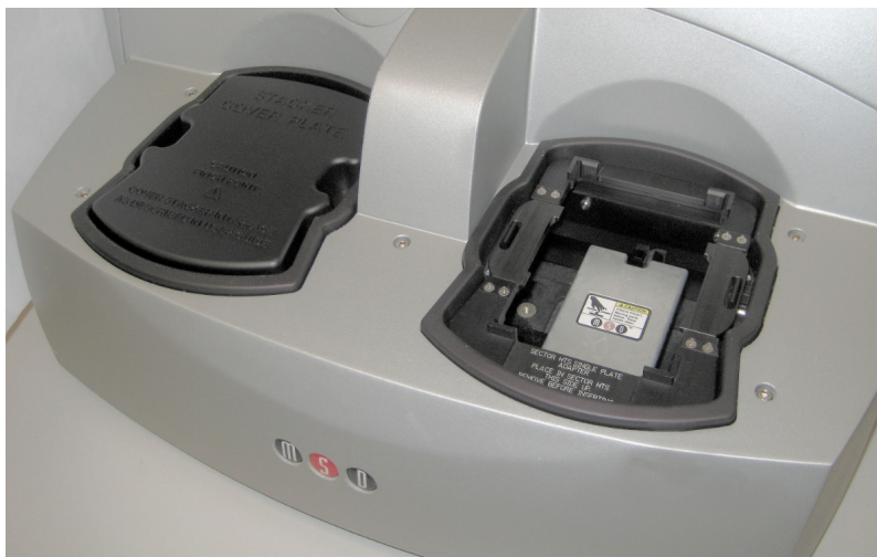
Figure 5:6 Stacker cover over the output port with empty single plate adaptor in the input port
