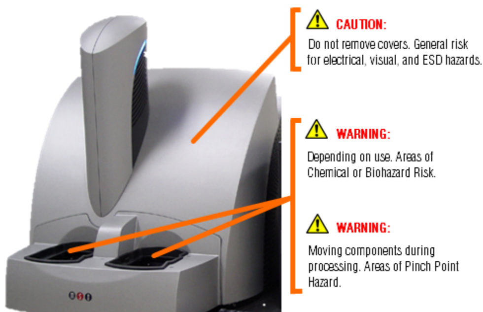
Figure 2:1 SECTOR S 600 electrical hazards.
